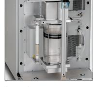
Optional recirculating nitrogen purge system reduces nitrogen consumption by  $\sim 1200\%$  annually
